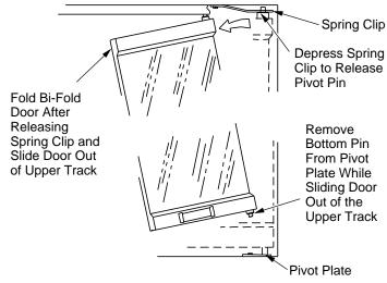
Figure 37 - Removing Glass Doors
